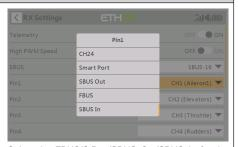
Select the FBUS/S.Port/SBUS Out/SBUS In for the channel ports.
